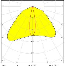
Dimensions: 50.0 mm x 50.0 mm Height: 10.60 mm ~20° + 115° oval beam for aisle lighting
