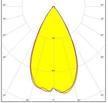
Dimensions: 50.0 mm x 50.0 mm Height: 8.50 mm ~50° wide beam optimized for CREE XP-L and XM-L
