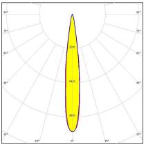
Dimensions: 50.0 mm x 50.0 mm Height: 10.00 mm ~10° spot beam. Variant made from PC.
