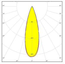
Dimensions: 50.0 mm x 50.0 mm Height: 8.50 mm ~25° medium beam. Variant made from PC.
