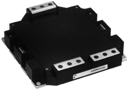
Dual switch (Half-Bridge)
