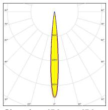
Dimensions: 37.8 mm x 37.8 mm Height: 24.08 mm ~10° spot beam with holder and installation tape
