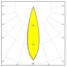
Dimensions: 37.5 mm x 37.5 mm Height: 24.08 mm ~25° wide beam with holder
