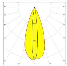
Dimensions: 37.8 mm x 37.8 mm Height: 24.10 mm ~12+40° oval beam with holder and installation tape
