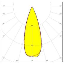
Dimensions: 37.5 mm x 37.5 mm Height: 24.17 mm ~35° spot beam with holder and installation tape
