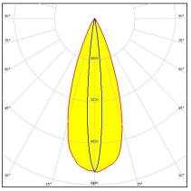
Dimensions: 37.8 mm x 37.8 mm Height: 24.29 mm ~12+40° oval beam with holder
