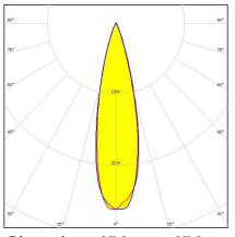
Dimensions: 37.8 mm x 37.8 mm Height: 24.08 mm ~25° spot beam with holder and installation tape
