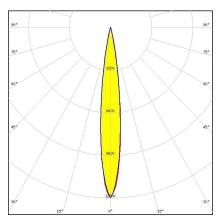
Dimensions: 37.8 mm x 37.8 mm Height: 24.08 mm ~10° spot beam with holder
