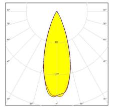
Dimensions: 37.5 mm x 37.5 mm Height: 24.17 mm ~35° wide beam with holder
