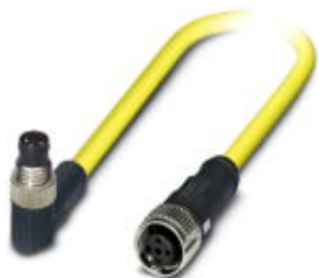
Sensor/actuator cable, 3-position, PVC, yellow, Plug angled M8, on Socket straight M12 SPEEDCON, A-coded, cable length: 0.5 m
