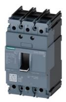
circuit breaker 3VA5 UL frame 125 breaking capacity class S 25kA @ 480 V 3-pole, line protection TM210, FTFM, In=70A overload protection Ir=70A fixed short-circuit protection Ii=10 x In UL489 SB (naval), 50 deg. cel. nut keeper kit on both sides
