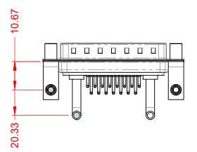
30A (CURRENT) **POWER/CO-AX CONTACT RATING:** (IF PRESENT) SIGNAL CONTACT CURRENT RATING: 5A PER CONTACT SIGNAL CONTACT RESISTANCE:  $10m\Omega$  MAX.
