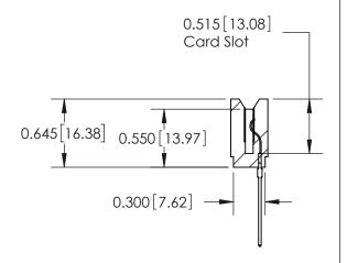
ACAD REFERENCE NO. 737 Series Ultra-Mate Card Edge Connector - Press Fit DRAWN: Part Number: 737-013-541-106 CHECKED: **EDAC INC** SCALE: THESE DRAWINGS AND SPECIFICATIONS ARE THE PROPERTY OF EDAC INC.,AND TORONTO, ONTARIO SHALL NOT BE REPRODUCED, OR COPIED DRAWING NUMBER CANADA OR USED AS THE BASIS FOR THE MANUFACTURE OR SALE OF APPARATUS YOUR CONNECTION TO QUALITY & SERVICE WITHOUT WRITTEN PERMISSION.
