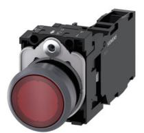
Illuminated pushbutton, 22 mm, round, plastic with metal front ring, red, pushbutton, flat, momentary contact type, with holder, 1 NO+1 NC, LED module with integrated LED 230 V AC, screw terminal, with laser labeling, upper case and lower case, Always upper case at the beginning of the word
