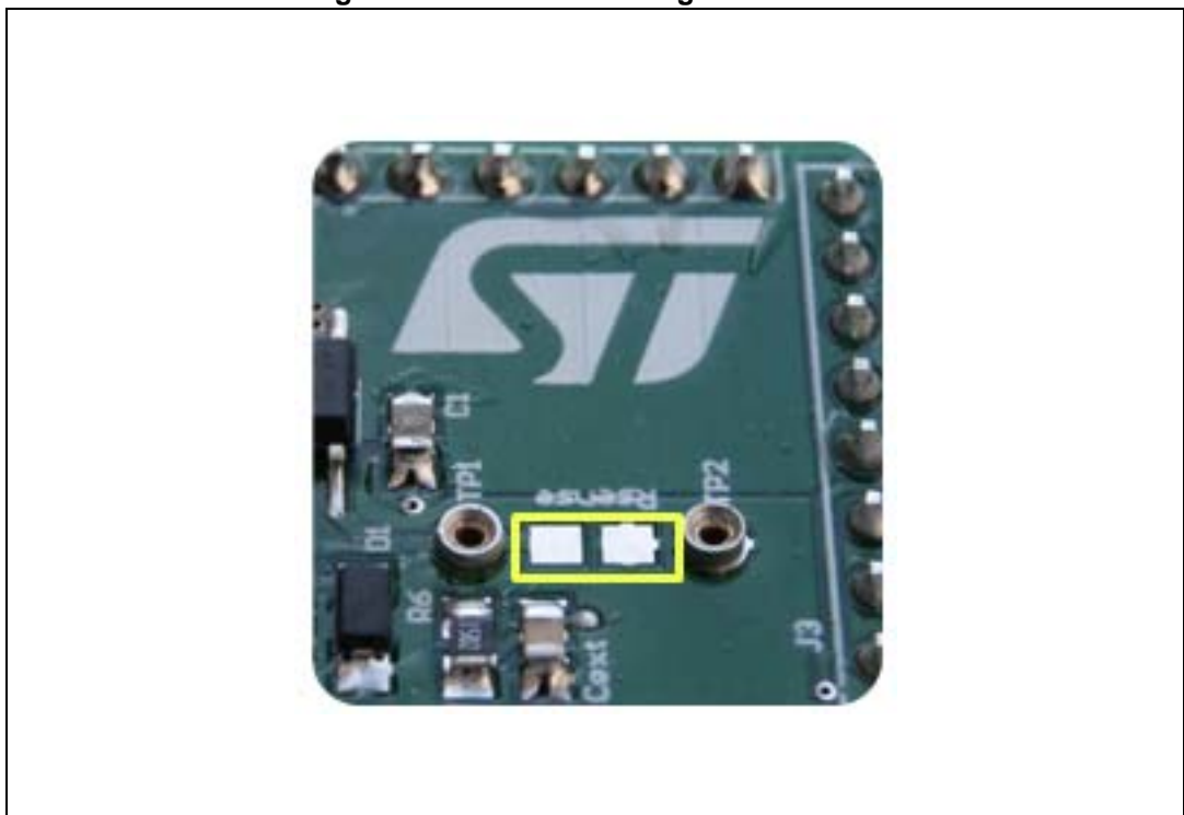
Figure 5. Pads for soldering SMD resistor
