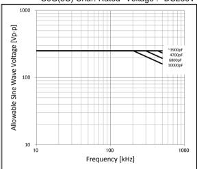
Except for 2012M/0805 and 3216M/1206 (2012M,3216M:Metric size code) C0G(5C) Char. Rated Voltage: DC250V
