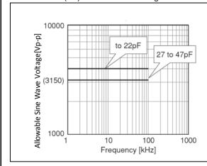
The capacitors less than 22pF can be applied maximum 4.0kV peak to peak at 100kHz or less only for the ballast or the resonance usage in the CFL inverter circuit.
