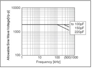
Frequency VS Allowable Sine Wave Voltage
