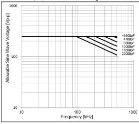
2012M/0805(2012M:Metric size code) C0G(5C) Char. Rated Voltage: DC250V
