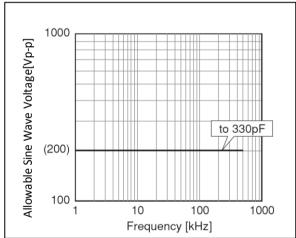
3216M/1206(3216M:Metric size code) C0G(5C) Char. Rated Voltage: DC250V
