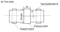
b:+/-5 gap between support stand center and test stand center
