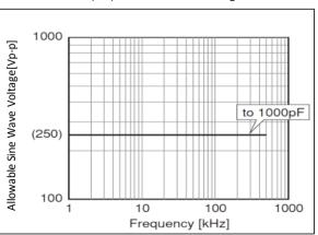
Frequency VS Allowable Sine Wave Voltage
