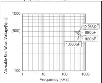
2012M/0805(2012M:Metric size code) C0G(5C) Char. Rated Voltage: DC630V
