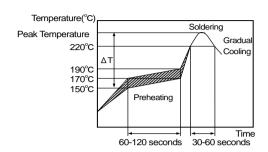
[Allowable Reflow Soldering Temperature and Time]
