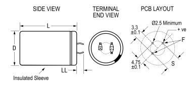
**General Information** Series PEH536 Dielectric Aluminum Electrolytic Description Snap-In, Aluminum Electrolytic RoHS Yes Lead 3 Pin Short AEC-Q200 No **Component Weight** 51 g Notes Add 0.5mm To D And 1mm To L For Sleeving. Shelf Life 208 Weeks
