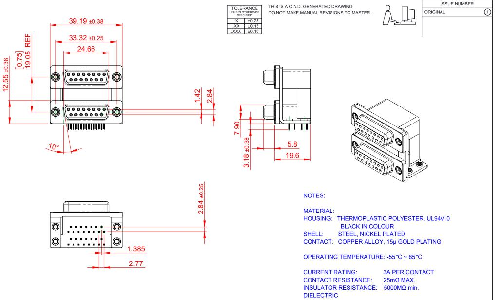
WITHSTANDING VOLTAGE: 1000V AC rms
