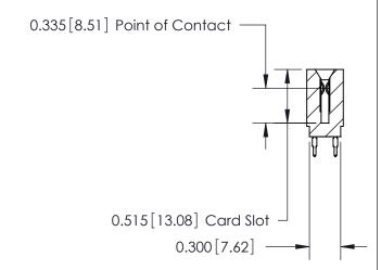
ACAD REFERENCE NO. 745 Series Ultra-Mate Card Edge Connector - Press Fit DRAWN: J.LEE Part Number: 745-038-525-201 CHECKED: **EDAC INC** SCALE: THESE DRAWINGS AND SPECIFICATIONS ARE THE PROPERTY OF EDAC INC., AND TORONTO, ONTARIO SHALL NOT BE REPRODUCED, OR COPIED DRAWING NUMBER CANADA OR USED AS THE BASIS FOR THE 745-ENG MASTER MANUFACTURE OR SALE OF APPARATUS YOUR CONNECTION TO QUALITY & SERVICE WITHOUT WRITTEN PERMISSION.
