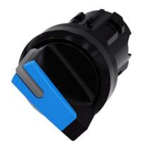
Selector switch, illuminable, 22 mm, round, plastic, blue, selector switch, short, 2 switch positions O<I, momentary contact type, Actuating angle 45°, 10:30h/12h, with laser labeling, upper case and lower case, always upper case at the beginning of the word
