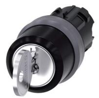
RONIS key-operated switch, 22 mm, round, plastic with metal front ring, lock number SB30, with 2 keys, 3 switch positions I-O<II, left latching, right momentary contact type, actuating angle 2x45°, 10:30h/12h/13:30h, key removal O+I, possible special locks: SB31, 421, 455, Z=50-unit packaging
