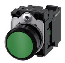
Pushbutton, 22 mm, round, plastic, green, pushbutton, flat, momentary contact type, with holder 1 NO, spring-type terminal, with laser labeling, upper case and lower case, always upper case at beginning of line
