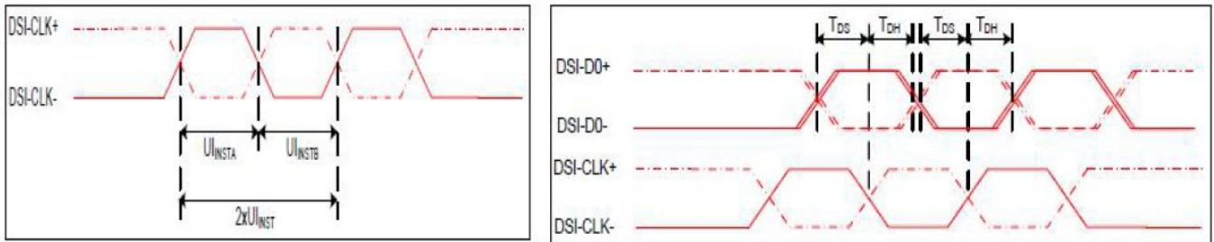
Figure 6.1: DSI Clock Channel Timing Diagram
