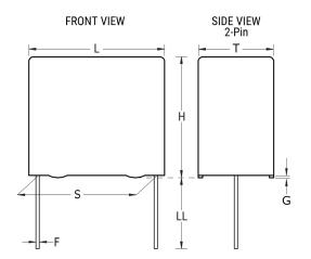
**General Information** Series F611 Dielectric Metallized Polyester Style Radial MKT (Wound), DC Multipurpose Applications Features RoHS Yes Lead Wire Leads AEC-Q200 No Component 23 g Weight The Rated Voltage Decreases 1.25%/C Between +85C And +105C (For +125C, Please Consult KEMET). ClimCat: 55/105/56. Miscellaneous
