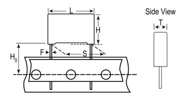
**General Information** Series R46 275 VAC Dielectric Metallized Polypropylene Style Radial EMI Safety Features RoHS Yes Lead Wire Leads Safety Class X2 ENEC, UL, cUL, CQC Qualifications AEC-Q200 No THB Performance No **Component Weight** 8.996 g We Recommended To Use R46 @ 310 VAC. Notes
