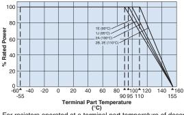
For resistors operated at a terminal part temperature of described for each size or above, a power rating shall be derated in accordance with derating curve. Please refer to "Introduction of the derating curves based on the terminal part temperature" in the beginning of our catalog before use.
