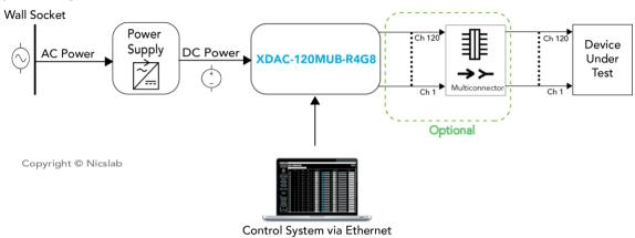
Figure 1. XDAC-120MUB-R4G8 System Diagram
