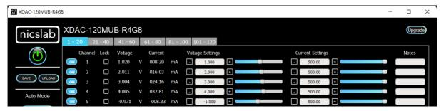
Note: When you upload CV mode, the current setting slider values automatically show 2184.50 bits to open the current flow from the supply. You may adjust this to match your requirements.
