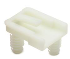
HellermannTyton Connector Clips provide a single method to mount connectors to various surfaces in a variety of applications. Highly engineered designs feature anti-rattle discs, anti-rotation oval fir trees and clamps for mounting on edges.
