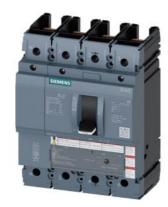
circuit breaker 3VA5 UL frame 250 breaking capacity class C 100kA @ 480V 4-pole, line protection TM230, FTAM, In=110A overload protection Ir=110A fixed short-circuit protection Ii=5...10 x In N conductor unprotected without connection
