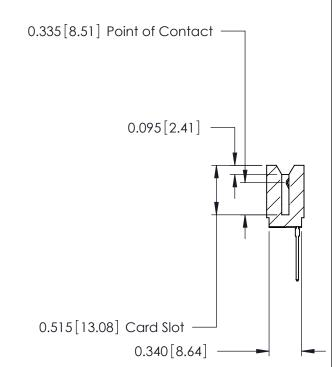
746 Series Ultra-Mate Card Edge Connector - Press Fit Part Number: 746-026-545-106
