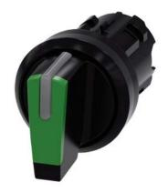
Selector switch, illuminable, 22 mm, round, plastic, green, selector switch, short, 3 switch positions I>O<II, momentary contact on the left, latching on the right, actuating angle 2x45°, 10:30h/12h/13:30h, with laser labeling, upper case and lower case, always upper case at the beginning of the word
