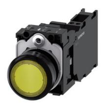
Illuminated pushbutton, 22 mm, round, plastic, yellow, pushbutton, flat, momentary contact type, with holder, 1 NO+1 NC, LED module with integrated LED 110 V AC, spring-type terminal, with laser labeling, upper case and lower case, Always upper case at the beginning of the word
