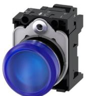
Indicator lights, 22 mm, round, metal, shiny, blue, lens, smooth, with holder, LED module with integrated LED 24 V AC/DC, spring-type terminal, with laser labeling, lower case
