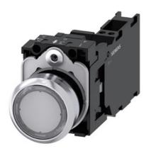
Illuminated pushbutton, 22 mm, round, metal, shiny, clear, pushbutton, flat, momentary contact type, with holder, 1 NO+1 NC, LED module with integrated LED 110 V AC, spring-type terminal, with laser labeling, upper case and lower case, Always upper case at the beginning of the word
