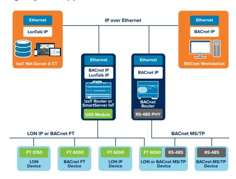
Designing a single system solution enables integrators to combine the strengths of the two most popular open building automation protocols, maximizing flexibility and improving results:
