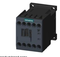
power contactor, AC-3 16 A, 7.5 kW / 400 V 1 NC, 600 V AC, 60 Hz 3-pole, Size S00 screw terminal
