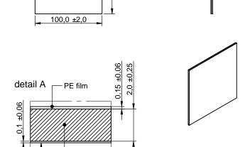
Silicone with ceramic particles
