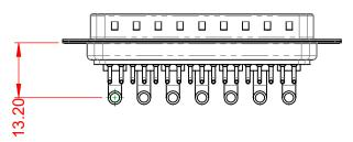
30A (CURRENT) POWER/CO-AX CONTACT RATING: (IF PRESENT) SIGNAL CONTACT CURRENT RATING: 5A PER CONTACT SIGNAL CONTACT RESISTANCE:  $10m\Omega$  MAX. INSULATOR RESISTANCE: 5000MΩ min.
