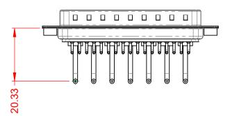
10A (CURRENT) POWER/CO-AX CONTACT RATING: (IF PRESENT) SIGNAL CONTACT CURRENT RATING: 5A PER CONTACT SIGNAL CONTACT RESISTANCE:  $10m\Omega$  MAX. **INSULATOR RESISTANCE:** 5000MΩ min. DIELECTRIC
