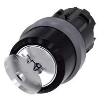
RONIS key-operated switch, 22 mm, round, plastic with metal front ring, lock number 455, with 2 keys, 2 switch positions O-I, latching, actuating angle 90°, 10:30h/13:30h, key removal O, Z=50-unit packaging
