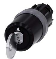
key-operated switch Siemens, 22 mm, round, plastic with metal front ring, lock number SSG10, with 2 keys, 3 switch positions I-O-II, latching, actuating angle 2x45°, 10:30h/12h/13:30h, key removal I+O+II, with laser labeling, lower case
