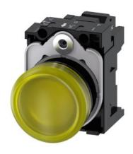
Indicator lights, 22 mm, round, plastic, yellow, lens, smooth, with holder, LED module, with integrated LED 24 V AC/DC, spring-type terminal, with laser labeling, upper case and lower case, always upper case at the beginning of the word
