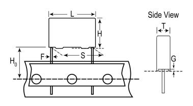
General Information Series F871 Dielectric Metallized Polypropylene Style Radial Features MKP EMI Safety RoHS Lead Wire Leads Safety Class X1 Qualifications ENEC, UL, cUL, CQC AEC-Q200 No THB Performance No Component Weight 2.104 g Miscellaneous ClimCat: 40/110/56/C. Shelf Life 104 Weeks
