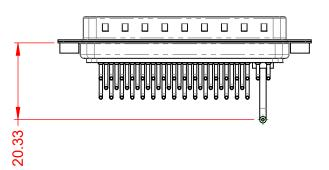
10A (CURRENT) POWER/CO-AX CONTACT RATING: (IF PRESENT) SIGNAL CONTACT CURRENT RATING: 5A PER CONTACT SIGNAL CONTACT RESISTANCE:  $10m\Omega$  MAX. **INSULATOR RESISTANCE:** 5000MΩ min. DIELECTRIC
