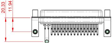
**OPERATING TEMPERATURE:** -55°C ~ 125°C POWER/CO-AX CONTACT RATING: 30A (CURRENT) (IF PRESENT) SIGNAL CONTACT CURRENT RATING: 5A PER CONTACT SIGNAL CONTACT RESISTANCE:  $10m\Omega$  MAX.
