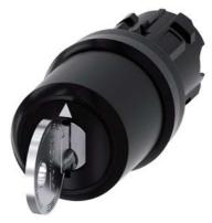
Key-operated switch IKON, 22 mm, round, plastic, special lock, with 2 keys, 3 switch positions I>O<II, momentary contact type, actuating angle  $2x45^\circ,\,10:30h/12h/13:30h,$  Key removal O
