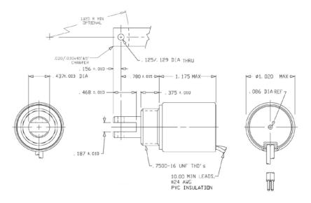
Solenoid shown energized with plunger fully seated Supplied with hex nut shipped loose Spring kits available (consult factory)
