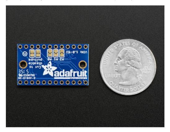
Using it is fairly straight-forward: the multiplexer itself is on I2C address 0x70 (but can be adjusted from 0x70 to 0x77)
