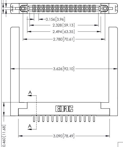
0.295[7.49] Card Slot **ECTION** 0.090 [2.29] Point of Contact 305 ENG MASTER 305 / 315 / 355 Card Edge Connector
