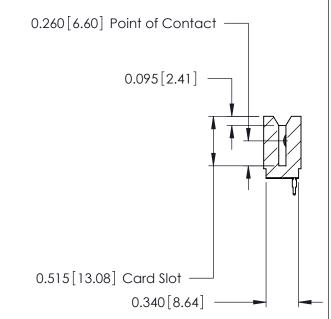
ACAD REFERENCE NO. 746 Series Ultra-Mate Card Edge Connector - Press Fit DRAWN: Part Number: 746-029-520-106 CHECKED: **EDAC INC** THESE DRAWINGS AND SPECIFICATIONS ARE THE PROPERTY OF EDAC INC.,AND TORONTO, ONTARIO SHALL NOT BE REPRODUCED, OR COPIED CANADA
