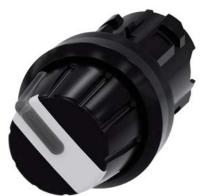
Selector switch, illuminable, 22 mm, round, plastic, white, Rotary knob, 2 switch positions O-I, latching, actuating angle  $90^{\circ}$ , 10:30h/13:30h, with laser labeling, upper case and lower case, always upper case at beginning of line
