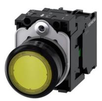
Illuminated pushbutton, 22 mm, round, plastic, yellow, pushbutton, flat, momentary contact type, with holder, 1NO, LED module with integrated LED 110 V AC, screw terminal, with laser labeling, upper case and lower case, Always upper case at the beginning of the word
