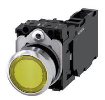
Illuminated pushbutton, 22 mm, round, metal, shiny, yellow, pushbutton, flat, momentary contact type, with holder, 1 NO+1 NC, LED module with integrated LED 110 V AC, screw terminal, Z=20-unit packaging
