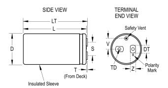
General Information Series ALS40 Dielectric Aluminum Electrolytic Description Screw Terminal, Aluminum Electrolytic RoHS AEC-Q200 No Halogen Free No Component 220 g Weight Dimensions D And L Include Sleeving. MS (MxH) = Notes M12x16. Mounting Clamp (Sold Separately): V4/2737 Shelf Life 156 Weeks
