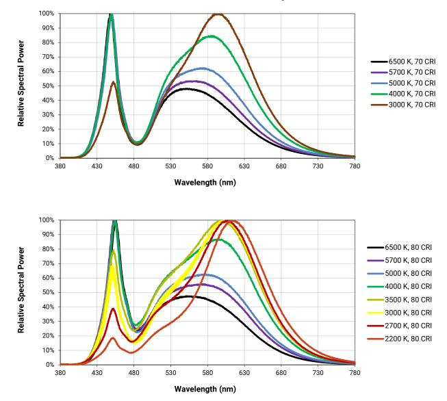
The following graphs are the result of a series of pulsed measurements at 600 mA and T<sub>1</sub> = 85 °C.
