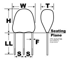
**General Information** Series T396 Dielectric MnO2 Tantalum Style **Radial Three Lead** Description Radial, Solid Tantalum, Three Leaded RoHS Yes Termination Tin AEC-Q200 No Construction Conformal Notes Longest Lead Is Positive.
